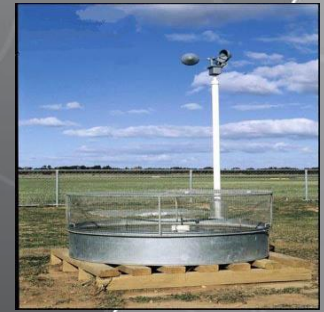
Class A Evaporation Pan
